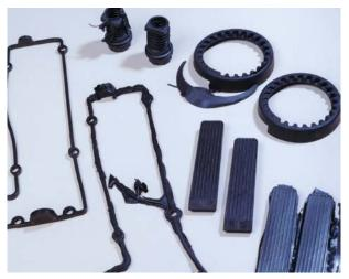
Rubber parts before and after deflashing
